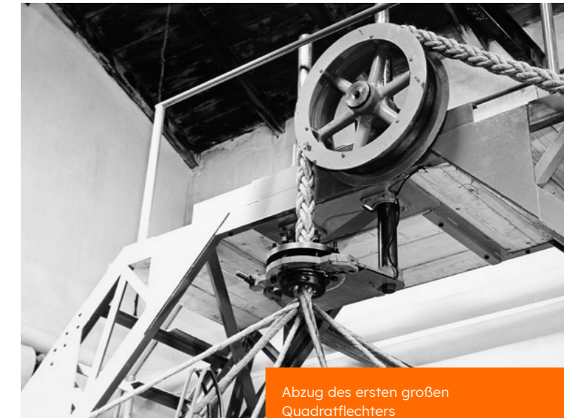
Pull-off unit of the first large square braider
